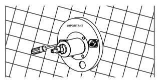
7. Proceed to aligne finish plate and install over the rough-valve.
