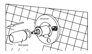
6. Turn on all stop valves and be sure to test the valve function before installing the finish plate.
