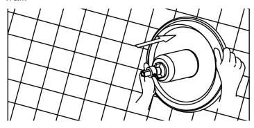
9. Align the handle and install it onto the valve. Secure handle in place with the provided setscrew.
