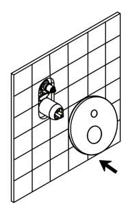
8. Align the handle and install it onto the valve. Secure handle in place with the provided setscrew.
