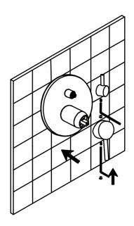
9. Proceed to connect the Shwoer Head and Bath Filler trim to the rough plumbing supply, and tighten firmly.
