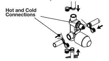
4. Connect the water supply outlets to the shower head and tub filler rough plumbing supply.
